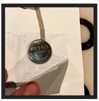
Next, tape down your conductive fabric tape over the lines you drew, carefully folding the tape to "turn" any corners. (The circuit works better if the tape is an unbroken line.)
