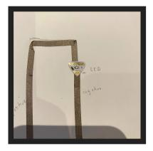
Once you have the positive and negative lines covered with the conductive tape, place your LED in the space you left, making sure that the positive and negative sides are in the correct place and that the metal pads of the LED are touching the conductive tape. Place the battery negative side down.
